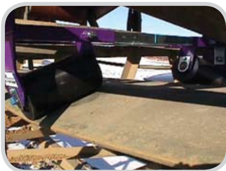
The Belt Positioner™ works on the belt's bottom cover so it will not cause any excessive wear or damage to the belt's edges.
