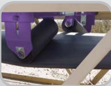
The Belt Positioner™ holds the belt in a centered position and influences the belt's path up to 100 feet (2.5 M) in both directions.
