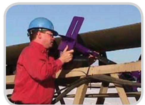
The Belt Positioner comes assembled and ready for quick installation.
